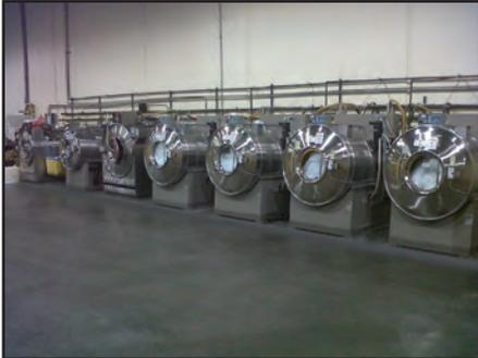
A single ozone system from this manufacturer handled all seven washers in use at the time, while other ozone systems for laundry handle only one or two washers each. The plant is processing at the rate of about 3,000,000 lbs/yr, operating seven days a week, with seasonal load variations calling for 8-12 hrs/day.
