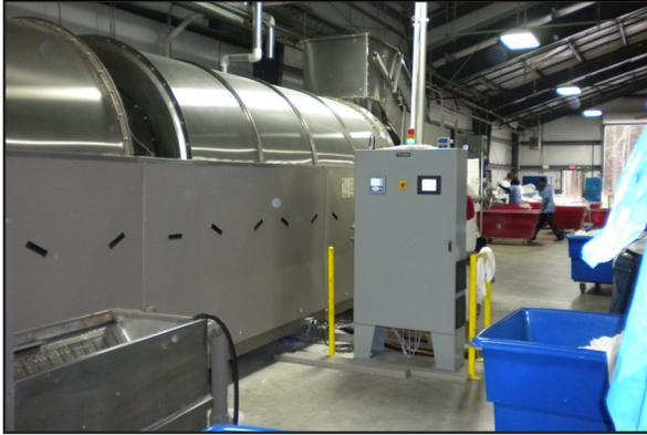
A small cabinet, 3-1/2 ft. wide x 6 ft. tall x 1 ft. deep, contains two ozone generators. The injection process features 24-hr. remote monitoring, data logging, and troubleshooting. The ozone system has sped up production by 10%, while increasing pounds per man hour by over 20%.
