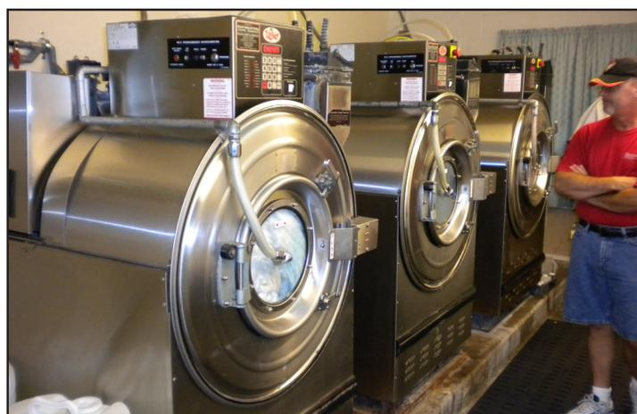
Ozone has allowed reductions in wash load steps and hot fills, as well as cuts in bleach and soap, and removal of softener.
