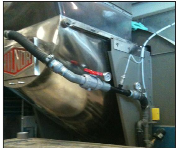
Ozonated water is injected directly into the wash wheel using a premium Venturi-type system that consistently provides mass transfer efficiency at the level of 90% or more.
